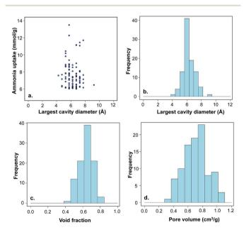
Fig. 8 Structure–property relationships derived for the top 97 MOF candidates with ammonia uptake greater than 6 mmol  $\rm g^{-1}$  at 100 000 Pa and 298 K. (a) Ammonia uptake  $\rm vs.$  largest cavity diameter. Histograms of structural properties of the top 97 MOFs are plotted for (b) largest cavity diameter, (c) void fraction, and (d) pore volume.
