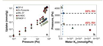
Fig. 3 (a) Simulated water adsorption isotherms for five MOFs studied at 298 K. (b) Water condensation pressures P<sub>i</sub> versus Henry's constants ( $K_{\rm H}$ ). The blue dashed line represents the  $K_{\rm H}=5\times10^{-6}$  mmol g<sup>-1</sup> Pa<sup>-1</sup> threshold criterion for hydrophobicity. Light green hexagons, FMOF-1; blue circles, ZIF-8; orange diamonds, Zn-pyrazole; green triangles, MIL-47; red squares, Al-NDC
