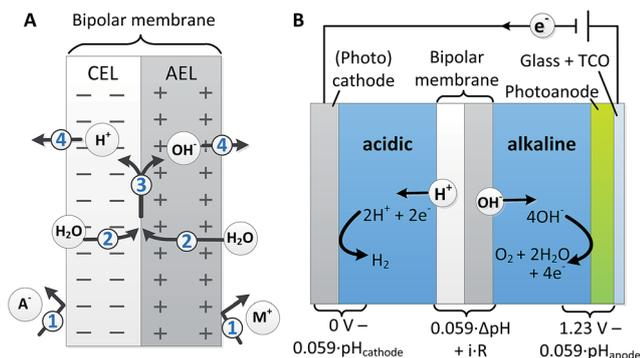
**Fig. 1** (A) Working principle of a bipolar membrane. Positive ions ( $M^+$ ) cannot enter the anion exchange layer (AEL) and negative ions ( $A^-$ ) cannot enter the cation exchange layer (CEL) (1). This results in water dissociation at the interface of these two layers (3), which is supplied by water diffusion (2) and leads to transport of  $H^+$  and  $OH^-$  (4). (B) An example of a bipolar membrane implemented in a solar fuel system, with 1 or possibly 2 photoelectrodes.
