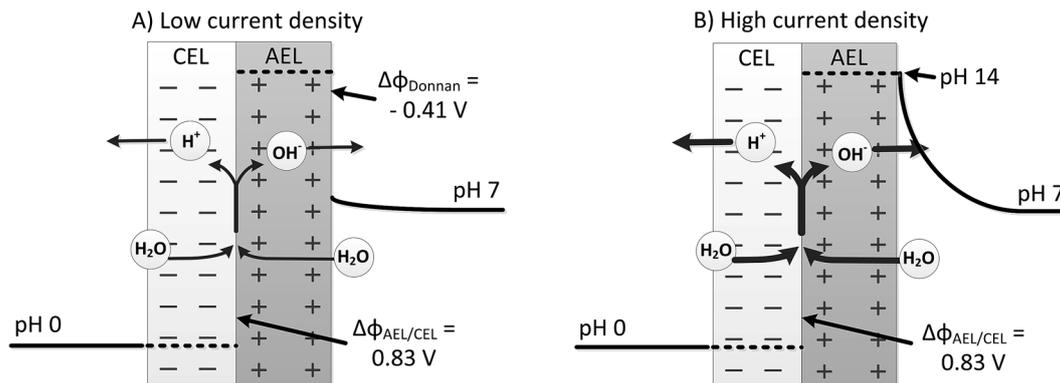
**Scheme 1** Bipolar membrane with internal (dotted line) and external (solid line) pH profiles, as hypothesized for low current density (A) and higher current density (B). The internal pH is assumed to be 0 in the cation exchange layer (CEL) and 14 in the anion exchange layer (AEL).
