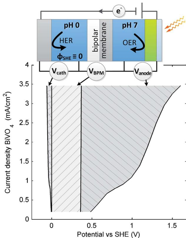
Fig. 3 Potential differences over the cathode ( $V_{\text{cath}}$ ), over the bipolar membrane ( $V_{\text{BPM}}$ ) and over the anode ( $V_{\text{anode}}$ ), obtained in the same configuration as for Fig. 2, except that the anode operates in pH 7 in this case. No correction for ohmic losses is applied.
