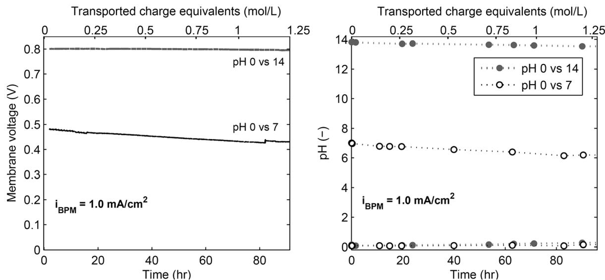
Fig. 5 Membrane voltage (left) and pH (right) as a function of time, at a constant current density of  $1 \text{ mA cm}^{-2}$  of BPM area (which corresponds to  $12.8 \text{ mA cm}^{-2}$  anode area in this case). Inert (Pt) electrodes were used as anode and cathode in this case.
