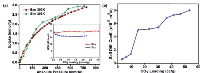
Fig. 6 (a) Comparison of the CO<sub>2</sub> isotherm simulated using the  $\alpha$ -phase and the experimental isotherm at 303 K. The inset shows the comparison of the HOA plots. (b) The self-diffusion coefficients of CO<sub>2</sub> in HPF-1 fitted using a spherical pore model.
