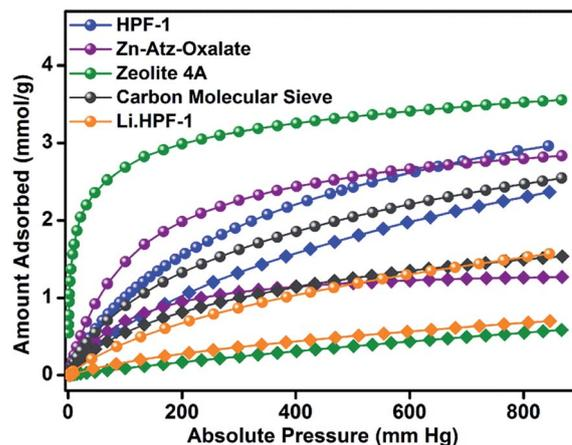
Fig. 4 Comparison of the effect of humidity on the CO<sub>2</sub> adsorption behavior of selected porous materials with varying hydrophobic-hydrophilic character and similar CO<sub>2</sub> uptakes. All isotherms were carried out at 303 K. *Important: after the steam conditioning the material was not subjected to any activation.* Note: spheres represent the activated phase; squares represent the steam conditioned phase.
