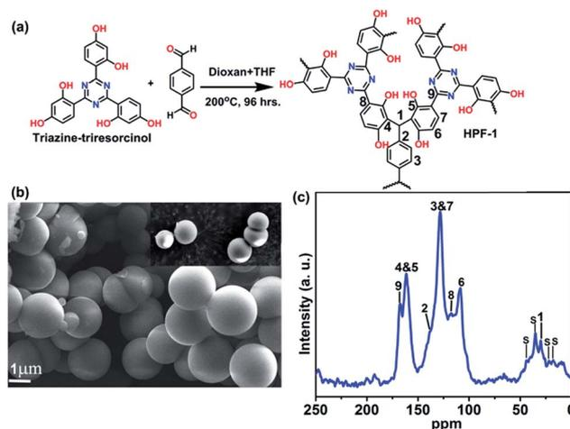
Fig. 1 (a) The reaction involved in the synthesis of HPF-1. (b) Microspheres formed by HPF-1 as seen from the FE-SEM image. (c) Shows the <sup>13</sup>C-MASNMR (400 MHz) of HPF-1, the peaks corresponding to the aromatic backbone and triazine groups can be observed. Few of the peaks in the aliphatic region correspond to the occluded THF and dioxane molecule in the polymer labelled as 's'.
