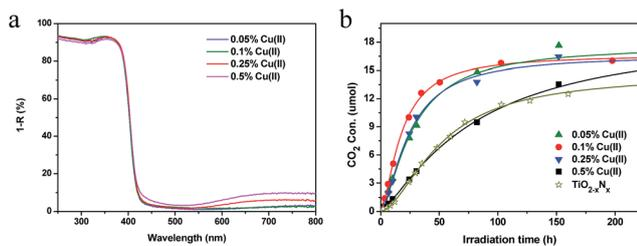
Fig. 5 (a) UV-Vis spectra for Cu(II)-TiO<sub>2</sub> samples with different amounts of grafted Cu(II) at pH 12 and (b) photocatalytic activities of the Cu(II)-TiO<sub>2</sub> samples in (a) and N-doped TiO<sub>2</sub> under visible-light irradiation.
