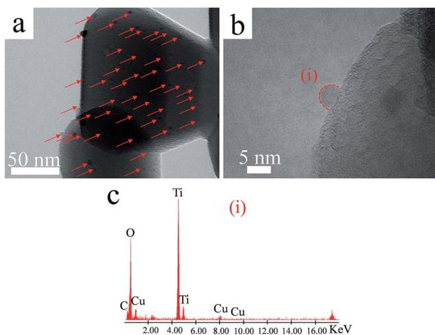
Fig. 2 (a) TEM and (b) HRTEM images of Cu(II)–TiO<sub>2</sub> (950-HCl-12). Nanoclusters (indicated by red arrows) were highly dispersed on the TiO<sub>2</sub> surface. In (b), the red dashed curve outlines a single Cu(II) nanocluster. The good attachment of nanoclusters and TiO<sub>2</sub> can be clearly observed. (c) EDS point analysis of the Cu(II) nanocluster on the point (i) in panel (b).
