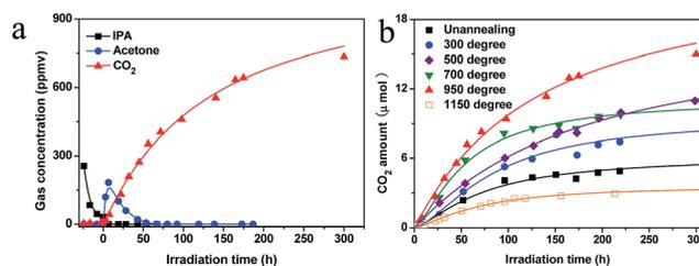
Fig. 3 (a) Representative time-dependent gas concentrations during IPA decomposition by the Cu(II)–TiO<sub>2</sub> (950-7) sample under visible-light irradiation. (b) Comparative analysis of CO<sub>2</sub> generation by Cu(II)–TiO<sub>2</sub> synthesized at different temperatures under the same conditions.
