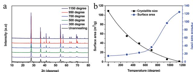
Fig. 1 (a) XRD patterns of TiO<sub>2</sub> samples obtained at various annealing temperatures and (b) crystallite sizes and surface areas of TiO<sub>2</sub> versus annealing temperature.
