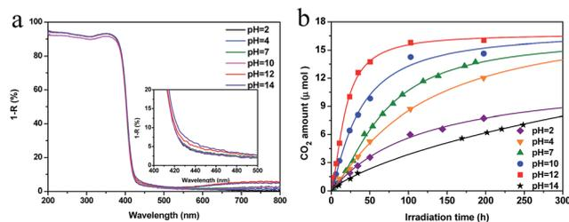
Fig. 4 (a) UV-Vis spectra for Cu(II)-TiO<sub>2</sub> (950-HCl) samples prepared at different pH values. (b) CO<sub>2</sub> generation curves for the prepared samples under visible-light irradiation.
