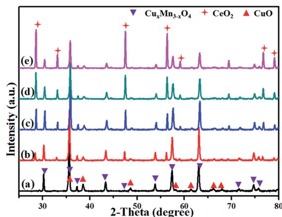
Fig. 5 XRD patterns after the TGA test from room temperature to 800 °C under flowing air: (a)  $\text{CuMnO}_2$ , (b)  $\text{CuMnO}_2-5\text{CeO}_2$ , (c)  $\text{CuMnO}_2-10\text{CeO}_2$ , (d)  $\text{CuMnO}_2-20\text{CeO}_2$ , and (e)  $\text{CuMnO}_2-40\text{CeO}_2$ .
