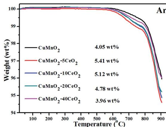
Fig. 7 TGA curves of oxidized  $\text{CuMnO}_2-x\text{CeO}_2$  samples (*i.e.*, after the TGA test up to 800 °C under flowing  $\text{O}_2$ ) from room temperature to 900 °C under flowing argon with 25  $\text{mL min}^{-1}$ .
