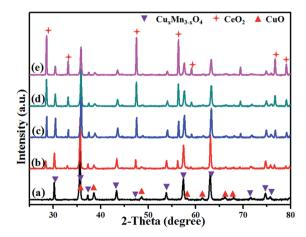
Fig. 5 XRD patterns after the TGA test from room temperature to 800 °C under flowing air: (a) CuMnO<sub>2</sub>, (b) CuMnO<sub>2</sub>–5CeO<sub>2</sub>, (c)  $CuMnO_2-10CeO_2$ , (d)  $CuMnO_2-20CeO_2$ , and (e)  $CuMnO_2-40CeO_2$ .
