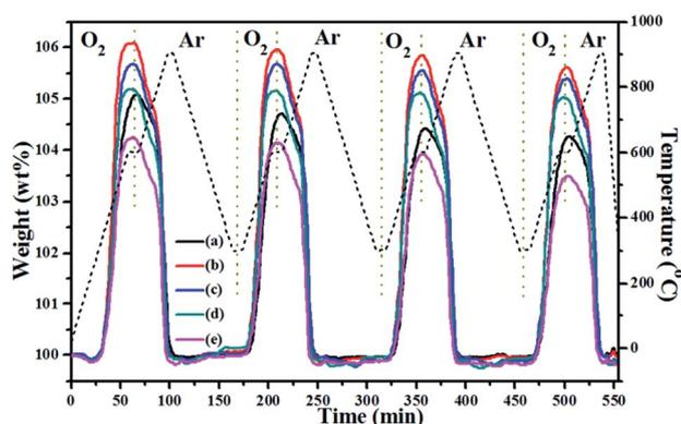
Fig. 8 TGA curves of the as-prepared  $\text{CuMnO}_2$ - $x\text{CeO}_2$  samples (*i.e.*, post-annealed at 960 °C for 12 h under flowing Ar) under alternating  $\text{O}_2$  and argon. The samples were first oxidized under  $\text{O}_2$  to 600 °C, then the gas was switched to argon and the temperature was increased to 900 °C. After being cooled down to 300 °C under argon, the gas was then switched back to  $\text{O}_2$  and oxidized to 600 °C.
