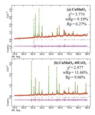
Fig. 3 XRD patterns after final Rietveld refinements for the asprepared products: (a)  $CuMnO_2$  and (b)  $CuMnO_2$ -40CeO<sub>2</sub>.
