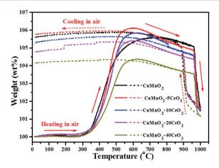
Fig. 6 TGA curves of the as-prepared CuMnO $_2$ -xCeO $_2$  samples (i.e., post-annealed at 960 °C for 12 h under flowing Ar) from room temperature up to 1000 °C with heating and cooling rates of 10 °C min $^{-1}$  under flowing air.
