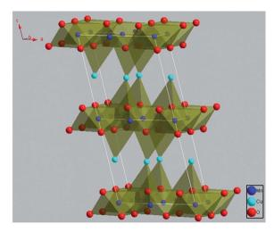
Fig. 1 Schematic illustration of the crystal structure of CuMnO<sub>2</sub>. The illustration was drawn with Diamond 3.1d software for crystal and molecular structure visualization.
