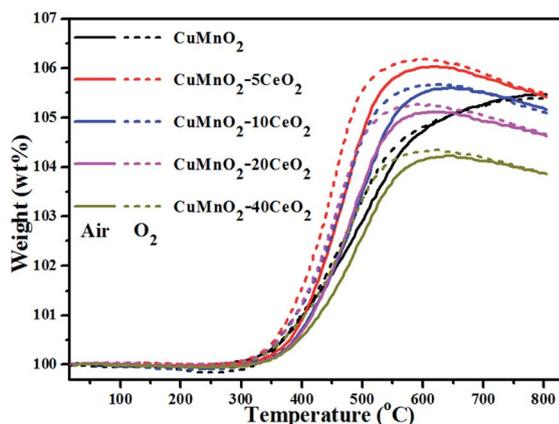
Fig. 4 TGA curves of the as-prepared  $\text{CuMnO}_2-x\text{CeO}_2$  samples (*i.e.*, post-annealed at 960 °C under flowing Ar for 12 h) under flowing air or pure  $\text{O}_2$  with  $25 \text{ mL min}^{-1}$  from room temperature to 800 °C. The solid lines are the TGA curves under air and the short dashed lines are the TGA curves under pure  $\text{O}_2$ .
