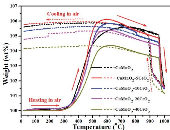
Fig. 6 TGA curves of the as-prepared  $\text{CuMnO}_2-x\text{CeO}_2$  samples (*i.e.*, post-annealed at 960 °C for 12 h under flowing Ar) from room temperature up to 1000 °C with heating and cooling rates of 10 °C  $\text{min}^{-1}$  under flowing air.
