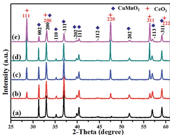
Fig. 2 XRD patterns of the as-prepared  $\text{CuMnO}_2-x\text{CeO}_2$  (i.e., post-annealed at 960 °C under flowing Ar): (a)  $\text{CuMnO}_2$ , (b)  $\text{CuMnO}_2-5\text{CeO}_2$ , (c)  $\text{CuMnO}_2-10\text{CeO}_2$ , (d)  $\text{CuMnO}_2-20\text{CeO}_2$ , and (e)  $\text{CuMnO}_2-40\text{CeO}_2$ .
