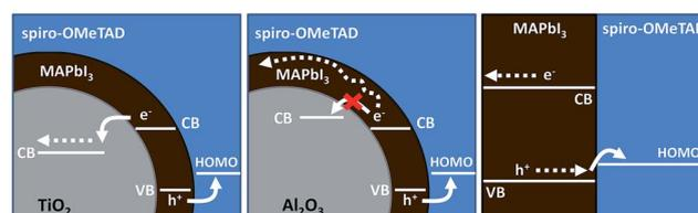
Fig. 1 Schematic to illustrate charge photogeneration in various device architectures incorporating MAPbI<sub>3</sub> as an absorber.
