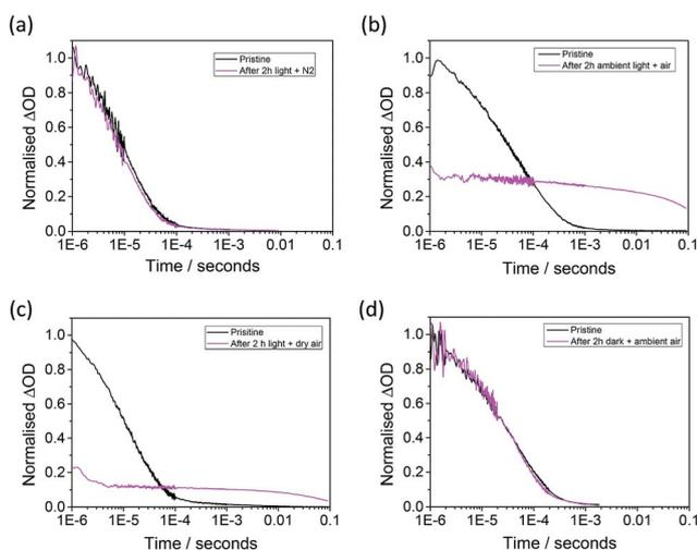
Fig. 4 Effect of exposure to varying environmental conditions for two hours on the transient absorption signal at 1600 nm for a mesoporous Al<sub>2</sub>O<sub>3</sub>/MAPbI<sub>3</sub>/spiro-OMeTAD film: (a) ambient light, sealed under flowing N<sub>2</sub>, (b) ambient light, non-sealed, (c) ambient light, sealed under flowing dry air (H<sub>2</sub>O < 2 vpm), (d) dark, non-sealed. Laser excitation energy density = 25  $\mu$ J cm<sup>-2</sup> at 567 nm.
