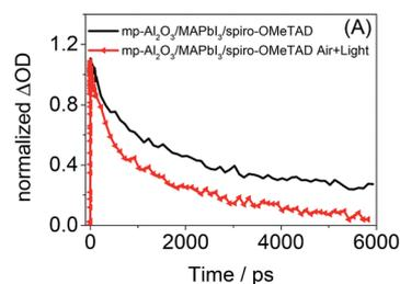
Fig. 5 Time-resolved transient absorption at 780 nm for pristine mp-Al<sub>2</sub>O<sub>3</sub>/MAPbI<sub>3</sub>/spiro-OMeTAD (black) and exposed to air and ambient light MAPbI<sub>3</sub>/spiro-OMeTAD (red) films. Traces normalized to  $\Delta OD = 1$  at 1 ps time-delay to highlight differences in recombination kinetics. Laser excitation energy density = 25  $\mu$ J cm<sup>-2</sup> at 567 nm.
