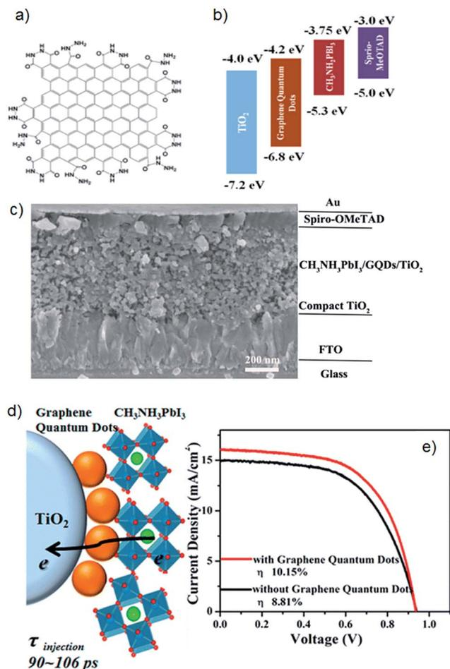
Fig. 8 (a) Schematic of GQD structure. (b) Energy levels of different layers used in PSCs of Zhu *et al.*<sup>81</sup> (c) Cross sectional SEM image of PSCs fabricated with GQDs. (d) Schematic illustration of electron generation and injection at the interfaces of TiO<sub>2</sub>, GQDs and perovskites. (e) Current density–voltage curves for the best performing PSCs. Reprinted with permission from ref. 81 © 2014, American Chemical Society.
