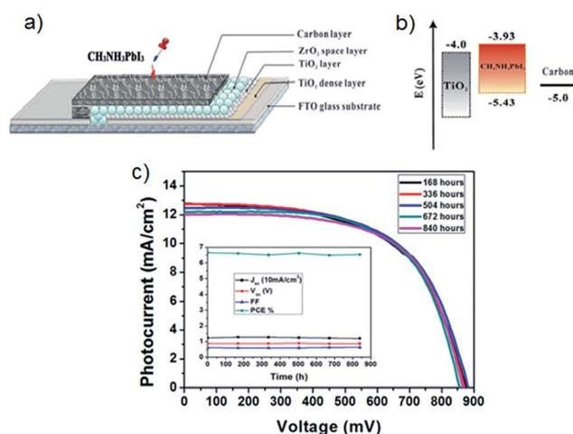
Fig. 4 (a) The structure of the first carbon counter electrode based PSC.<sup>64</sup> (b) Energy level of  $\text{TiO}_2$ ,  $\text{CH}_3\text{NH}_3\text{PbI}_3$  and carbon.<sup>64</sup> (c) Current density–voltage curves of carbon cathode based PSCs over 840 hours. Inset: the effect of time on each value ( $J_{sc}$ ,  $V_{oc}$ , FF and PCE) of solar cell. Reprinted with permission from ref. 64 © 2013, Nature Publishing Group.
