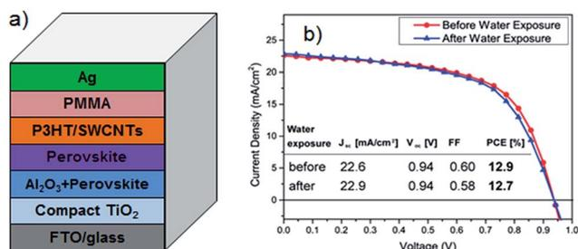
Fig. 6 (a) Schematic illustration of PSC fabricated with CNTs/polymer composite as a hole collection layer as reported by Snaith's group.<sup>79</sup> (b) Current density–voltage curves of PSCs before and after water exposure for 60 s (reprinted with permission from ref. 79 © 2014, American Chemical Society).
