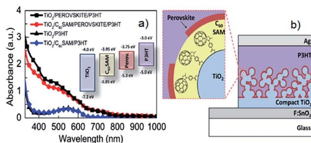
Fig. 7 (a) UV-vis spectra of P<sub>3</sub>HT and perovskite films with and without C<sub>60</sub>SAM. Inset: the energy level of the components used in Snaith's work.<sup>85</sup> (b) The structure of the PSC fabricated with C<sub>60</sub>SAM layer between perovskite and TiO<sub>2</sub> layers. Reprinted with permission from ref. 85 © 2013, American Chemical Society.
