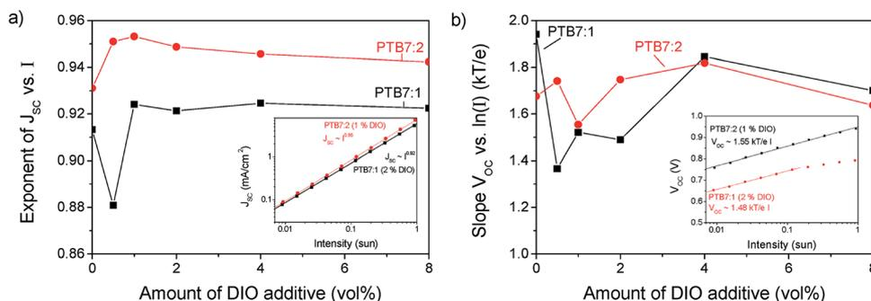
Fig. 8 (a) The exponent of the short circuit density vs. light intensity ( $I$ ) as a function of content of DIO. The inset shows an example at the optimized conditions. (b) Slope of the open circuit voltage as a function of content of DIO. The inset shows an example at the optimized conditions.
