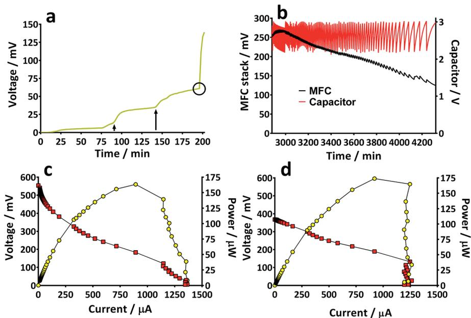
Fig. 6 Performance of TP-MFC stack when connected to power management system; (a) inoculant introduced at  $t = 0$ , arrows show when MFCs were topped up with additional inoculant, circle highlights point when working voltage became high enough to kick-start PMS; (b) stack and capacitor charge/discharge cycle during day 3; (c) power and polarisation curves on day 5; (d) power and polarisation curves on day 61.
