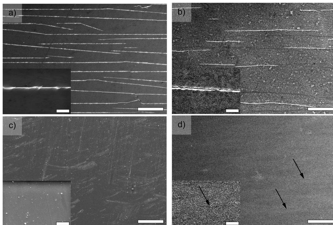
Fig. 4 Low-magnification (main) and high-magnification (inset) SEM images of: (a) PET/M-In<sub>2</sub>O<sub>3</sub>, (b) PET/M-In<sub>2</sub>O<sub>3</sub>/ZnO/CH<sub>3</sub>NH<sub>3</sub>PbI<sub>3</sub>, (c) PET/HC-PEDOT, and (d) PET/HC-PEDOT/SC-PEDOT/CH<sub>3</sub>NH<sub>3</sub>PbI<sub>3</sub> films after 2000 bending cycles. The scale bars in the main and inset images are 50 μm and 5 μm, respectively. The arrows in (d) show the location of small cracks in the perovskite layer.
