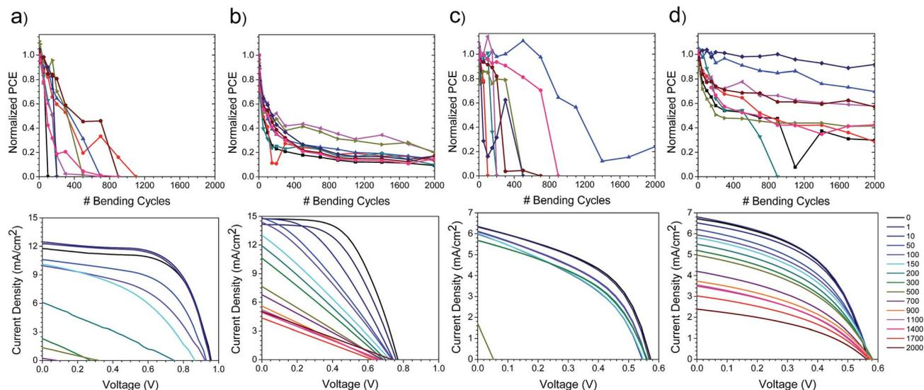
Fig. 3 Results of the fatigue tests for the (a) M-In<sub>2</sub>O<sub>3</sub>/ZnO/CH<sub>3</sub>NH<sub>3</sub>PbI<sub>3</sub>, (b) HC-PEDOT/SC-PEDOT/CH<sub>3</sub>NH<sub>3</sub>PbI<sub>3</sub>, (c) M-In<sub>2</sub>O<sub>3</sub>/ZnO/P3HT:PC<sub>61</sub>BM, and (d) HC-PEDOT/SC-PEDOT/P3HT:PC<sub>61</sub>BM devices. The top row shows the normalized PCE for each of 9 separate devices. The bottom row shows the *J*-*V* curves as a function of the number of bending cycles for a typical device.
