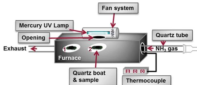
Fig. 1 A horizontal CVD furnace with a mercury UV lamp housing equipped with a cooling fan system. Position 1 is the position where  $\text{NH}_3$  was irradiated but the quartz boat and its contents were not irradiated by UV-light. Position 2 marks the position where the  $\text{NH}_3$ , the quartz boat and its contents are illuminated by the UV-light.
