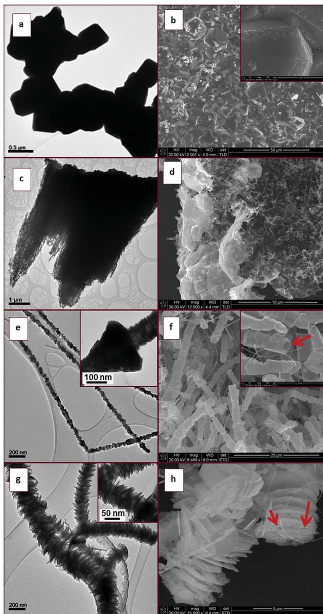
**Fig. 2** (a) TEM and (b) SEM images of as purchased  $\text{In}_2\text{O}_3$  particles, (c) TEM and (d) SEM images of perforated materials formed at  $700^\circ\text{C}$ , (e) TEM and (f) SEM images of segmented rod like structures at  $750^\circ\text{C}$  (the arrow indicates the hollow core), (g) TEM and (h) SEM images of flaky structures at  $800^\circ\text{C}$  (the arrows show perforations). All reactions were performed by photolysis of  $\text{NH}_3$  only.
