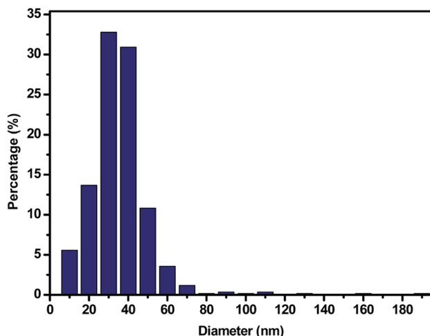
Fig. 9 InN nanotube diameters obtained from TEM studies.
