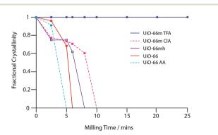
Fig. 4 Analysis of the crystallinity for various modulated UiO-66 samples as a function of milling time (TFA = trifluoroacetic acid; CIA = chloroacetic acid; AA = acetic acid, mh = modulated removed by heating). Fractional crystallinity is calculated from starting integral breadth/integral breadth at time t.
