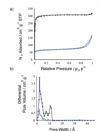
Fig. 3 (a) Nitrogen sorption isotherms at 77 K for UiO-66m TFA (dark blue) and UiO-66m TFA after 25 minutes of ball-milling (light blue). Open symbols – desorption, closed symbols – adsorption. (b) Pore size distributional analysis for crystalline (dark blue) and partially amorphized (light blue) UiO-66m TFA after 25 min milling.
