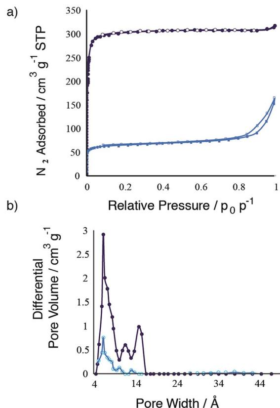
Fig. 3 (a) Nitrogen sorption isotherms at  $77$  K for UiO-66m TFA (dark blue) and UiO-66m TFA after 25 minutes of ball-milling (light blue). Open symbols – desorption, closed symbols – adsorption. (b) Pore size distributional analysis for crystalline (dark blue) and partially amorphized (light blue) UiO-66m TFA after 25 min milling.
