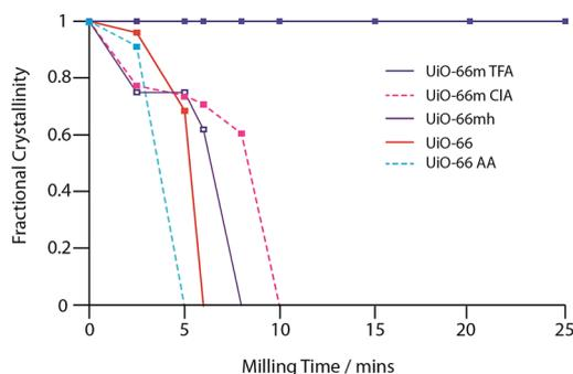
**Fig. 4** Analysis of the crystallinity for various modulated UiO-66 samples as a function of milling time (TFA = trifluoroacetic acid; CIA = chloroacetic acid; AA = acetic acid, mh = modulated removed by heating). Fractional crystallinity is calculated from starting integral breadth/integral breadth at time *t*.
