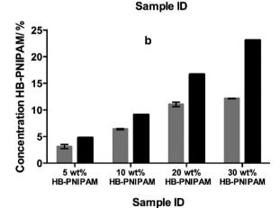
Fig. 2 Composition (determined by FTIR spectroscopy) of the networks prior to and after Soxhlet extraction with 2-propanol: (a) 10 wt% DEGDA in the monomer feed and (b) 40 wt% DEGDA in the monomer feed. The grey columns show the percentage of HB-PNIPAM in the BS-IPNs after extraction and the black columns show the percentage of HB-PNIPAM in the feeds. The spectral region used for analysis was 1480-1760 cm<sup>-1</sup>.
