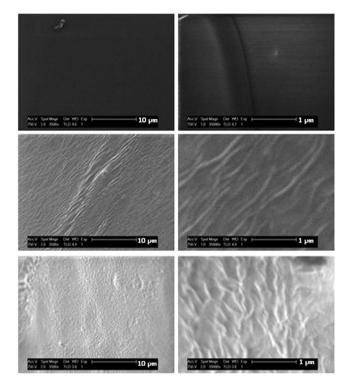
Fig. 4 High resolution electron micrographs of polymer surfaces  $\times 3500$  (left column),  $\times 35\,000$  (right column).The images show X-PVP hydrogel (top row), 10% HB-PNIPAM/X-PVP S-IPN (central row), 20% HB-PNIPAM/X-PVP S-IPN (bottom row). Left column shows SEM images at  $\times 35\,00$  magnification with 10  $\mu m$  scale bars, the right column shows SEM images at  $\times 35\,000$  magnification with 1  $\mu m$  scale bars.
