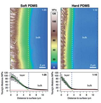
Fig. 4 Peak Force QNM analysis: the terrain images are nanomechanical mappings of the Young's modulus at the bulk/oxide layer interphase of soft (left) and hard PDMS (right). Below are the according cross section profiles that were averaged over the whole image size consisting of 469 lines.
