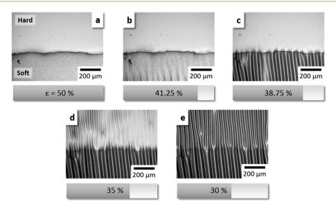
Fig. 3 Same-spot in situ observation of the release process, focused on the crossover line from hard to soft PDMS. The soft discrete inclusion is present at the bottom each, the hard at the top. In the beginning the substrate is pre-strained to 50% of its initial length (a), the oxidized layer on top is unstrained. Upon strain release wrinkles do form first within the soft inclusion (b and c) followed by the hard matrix (d and e). For a video capture of this process, see ESI.†
