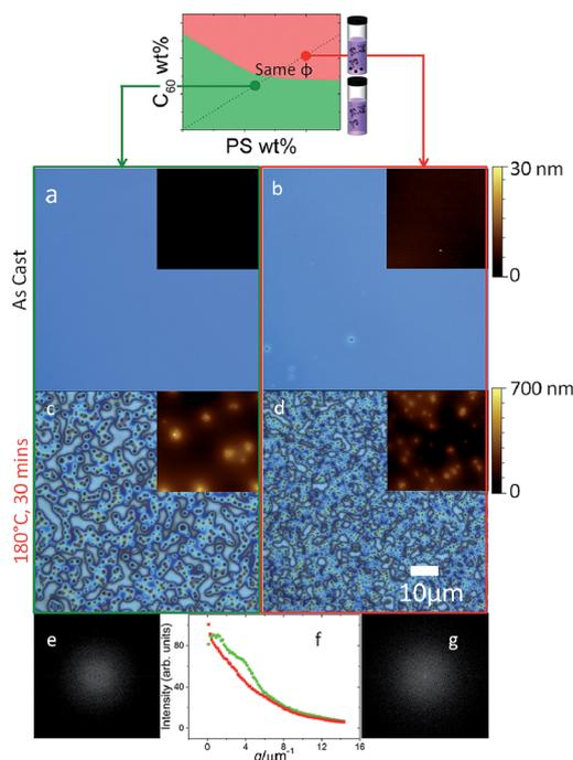
Fig. 4 Effect of thermal annealing (180 °C, 30 min) on the morphology of spun cast 5%  $C_{60}$ /PS 130 nm thin films prepared from solutions in the (a and c) homogeneous and (b and d) precipitated regimes. FFTs of (c) and (d) are shown in (e) and (g), respectively, whose radial profiles are compared in (f). Insets in (a–d) show AFM scans of the corresponding films, with an image width of 10  $\mu\text{m}$ ; the height scale bars are 30 nm in (a and b) and 700 nm in (c and d).
