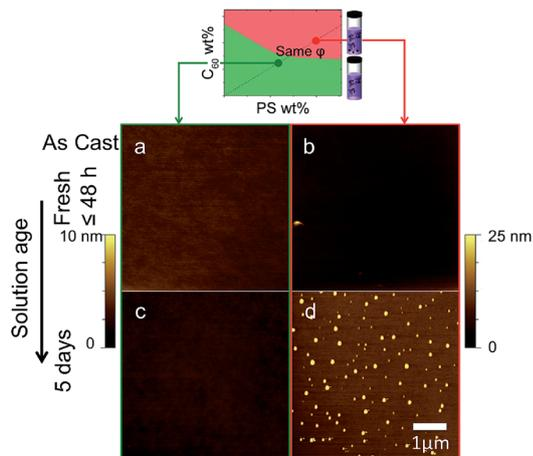
Fig. 3 Effect of solution age on spun cast thin films, across the miscibility boundary. AFM topography images of 5%  $C_{60}$ /PS 130 nm as-cast thin films prepared from (a and b) a freshly made solution and (c and d) a solution aged for 5 days.
