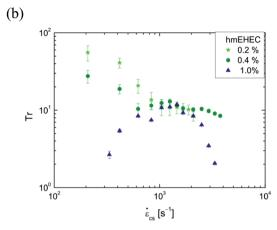
Fig. 7 Cross-slot extensional rheometry for hmEHEC solutions. (a) Extensional viscosity and (b) Trouton ratio as a function of imposed strain rate, determined from pressure drop measurements in the cross-slots for three hmEHEC solutions.
