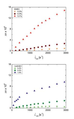
Fig. 4 Flow birefringence as a function of imposed strain rate, measured in the cross-slot extensional rheometer. Top: EHEC dispersion, bottom: hmEHEC dispersions.
