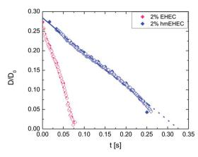
**Fig. 9** Capillary thinning analysis of 2 wt% cellulose ether solutions. Diameter *vs.* time measured using a laser micrometer is shown in filled symbols for 2% EHEC solution and 2% hmEHEC solution. The open symbols represent diameter *vs.* time data obtained from image analysis.
