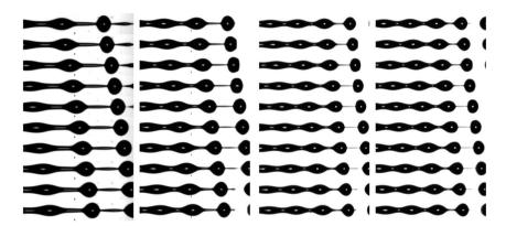
Fig. 11 Jet breakup of 0.225% hmEHEC. The forcing frequency in each column is  $kR_0 = 0.52$  (3.1 kHz),  $kR_0 = 0.67$  (4.05 kHz),  $kR_0 = 0.75$  (4.5 kHz) and  $kR_0 = 0.82$  (4.90 kHz) respectively, and  $\Delta f = 0.1$  Hz. Each panel has 10 images, each separated by 20  $\mu$ s. Note here Oh = 0.025, We = 40, and Re = 160.
