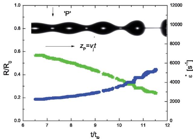
Fig. 12 Jetting analysis of 0.23% hmEHEC solution showing scaled radius  $R(t)/R_0$  vs. scaled time for Langragian point 'P' on the thinning neck (green symbol, left axis). The forcing frequency is  $kR_0 = 0.78$ . The blue circles on the right hand axis show the extension rate (see eqn (6)) as a function of scaled time.
