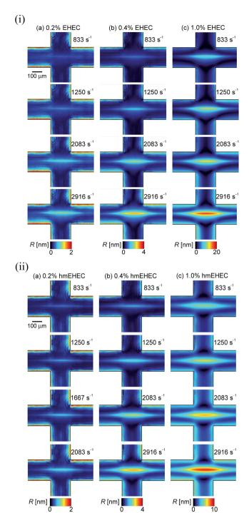
Fig. 3 (i) Birefringence in EHEC aqueous solutions in a cross-slot flow at the extensional rates indicated. Scale bar represents (a) 0-2 nm, (b) 0-4 nm, and (c) 0-20 nm. (ii) Birefringence in hmEHEC aqueous solutions in a cross-slot flow at the extensional rates indicated.
