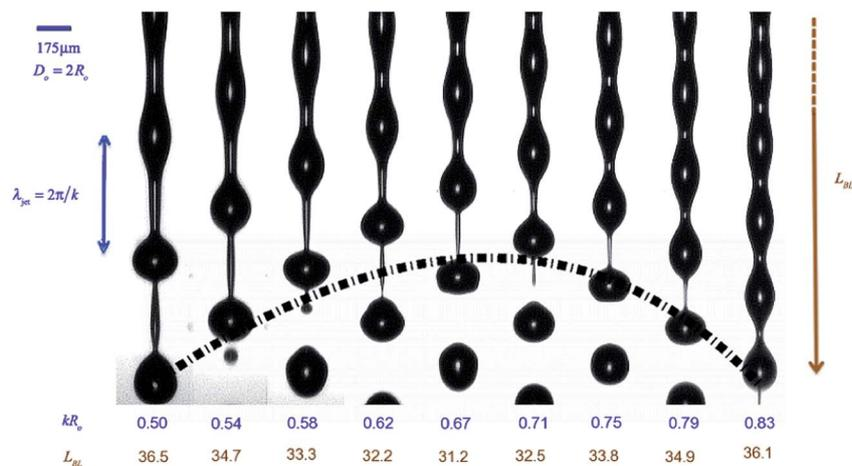
Fig. 10 Forced jetting of 0.23% hmEHEC solutions. The imposed perturbation frequency ( $kR_0$ ) is varied using an annular piezoelectric transducer. The black, dotted line shows the break-up length expected on the basis of linear stability analysis for inviscid fluid. The jet is backlit, and it refracts light away from the image plane causing the jet and drops to appear dark, except at the very center where light passes straight through the jet towards the camera.
