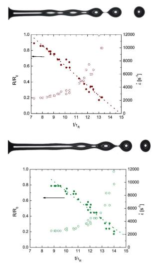
Fig. 14 Neck radius vs. time comparison of 0.4% EHEC & 0.4% hmEHEC solutions, obtained by analyzing ROJER data. The data are based on images acquired using the JetXpert system.
