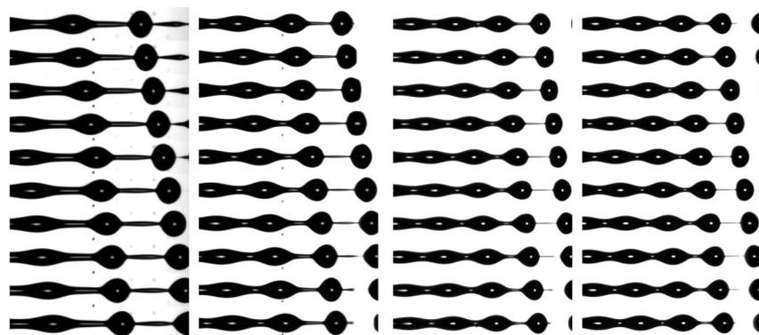
Fig. 11 Jet breakup of 0.225% hmEHEC. The forcing frequency in each column is  $kR_0 = 0.52$  (3.1 kHz),  $kR_0 = 0.67$  (4.05 kHz),  $kR_0 = 0.75$  (4.5 kHz) and  $kR_0 = 0.82$  (4.90 kHz) respectively, and  $\Delta f = 0.1$  Hz. Each panel has 10 images, each separated by 20  $\mu\text{s}$ . Note here  $\text{Oh} = 0.025$ ,  $\text{We} = 40$ , and  $\text{Re} = 160$ .
