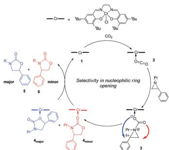
**Intramolecular ring-opening from a CO<sub>2</sub>-derived nucleophile as the origin of selectivity for 5-substituted oxazolidinone from the (salen)Cr-catalyzed [aziridine + CO<sub>2</sub>] coupling**
