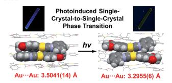
Photoinduced single-crystal-to-single-crystal phase transition and photosalient effect of a gold(1) isocyanide complex with shortening of intermolecular aurophilic bonds
