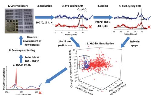
**Proxy-based accelerated discovery of Fischer–Tropsch catalysts**
