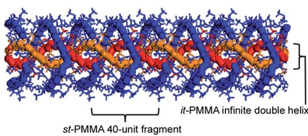
**Molecular mapping of poly(methyl methacrylate) super-helix stereocomplexes**
