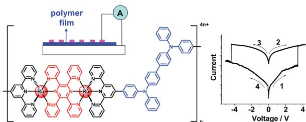
**Tuning of resistive memory switching in electropolymerized metallopolymeric films**
