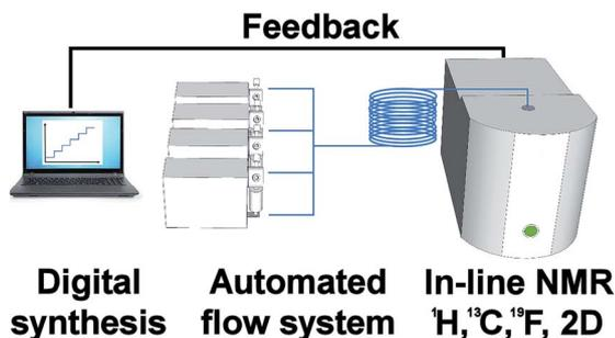
**A self optimizing synthetic organic reactor system using real-time in-line NMR spectroscopy**
