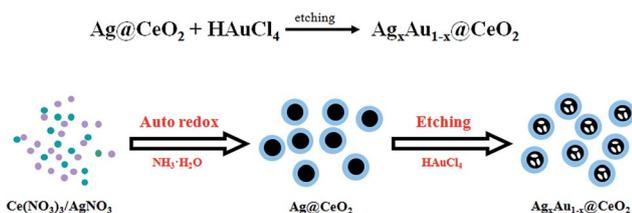
Scheme 1 Synthetic strategy for  $\text{Ag}_x\text{Au}_{1-x}@CeO_2$  core@shell nanospheres.
