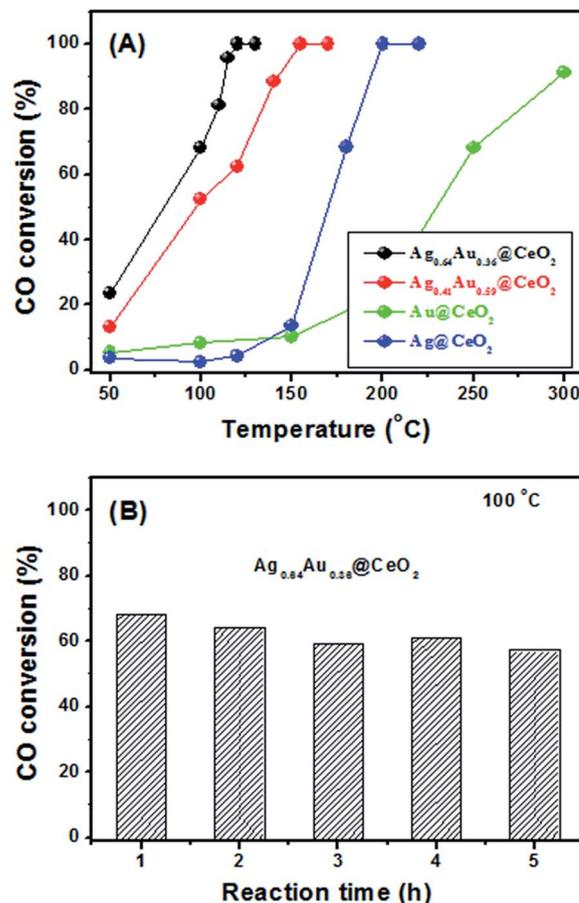
Fig. 4 (A) CO conversion curves of  $\text{Ag}@CeO_2$ ,  $\text{Ag}_{0.64}\text{Au}_{0.36}@CeO_2$ ,  $\text{Ag}_{0.41}\text{Au}_{0.59}@CeO_2$  and  $\text{Au}@CeO_2$ ; (B) cycling test of  $\text{Ag}_{0.64}\text{Au}_{0.36}@CeO_2$  at  $100 \text{ }^\circ\text{C}$  for 5 h.
