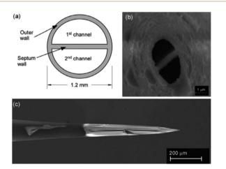
Fig. 3 Theta-shaped profile of glass capillary (a) sketch of the distal end and (b) electron micrograph of the very tip of a sputter-coated emitter and (c) electron micrograph of the side of the emitter showing hand-painted platinum-coating to the left of the tip. Copyright 2012 IM Publications. Reproduced with permission from ref. 42.
