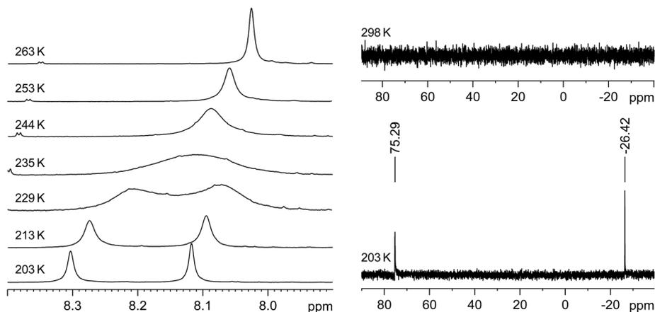
Fig. 4 Left: Excerpts of the variable-temperature  $^1\text{H}$  NMR (300.1 MHz) spectra of  $3 \cdot (\text{C}_6\text{H}_5\text{F})$  in  $\text{THF-}d_8$  in the temperature range 203–263 K showing the coalescence of the  $\text{C}^{4,5}\text{-H}$  signals. Right:  $^{29}\text{Si}\{^1\text{H}\}$  NMR (59.63 MHz) spectra of  $3 \cdot (\text{C}_6\text{H}_5\text{F})$  in  $\text{THF-}d_8$  at 203 K (bottom) and 298 K (top).
