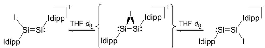
Scheme 3 Topomerisation of  $[\text{Si}_2(\text{I})(\text{Idipp})_2]^+$  occurring in solution. The tentative intermediate, a NHC-stabilised disilaidonium ion, is depicted in curly brackets. Formal charges are omitted for simplicity.
