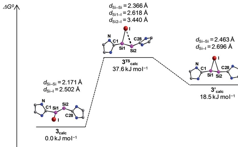
Fig. 5 Schematic Gibbs energy profile ( $T = 298$  K) for the degenerate isomerisation of the cation  $[\text{Si}_2(\text{I})(\text{Idipp})_2]^+$ , including the optimized minimum structures  $3_{\text{calc}}$  and  $3'_{\text{calc}}$  and the transition state  $3^{\text{TS}}_{\text{calc}}$  with selected bonding parameters. The N-bonded dipp substituents are omitted for clarity and only one half of the symmetric energy profile is depicted.
