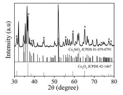
Fig. 3 XRD pattern of the nanobelts@ $Co_3O_4$  nanoparticles after annealing in air at 800 °C. The reflections marked with asterisks can be assigned to  $Co_3O_4$  (JCPDS 42-1467). All other reflections match with  $Co_2SiO_4$  (JCPDS 01-079-0791).
