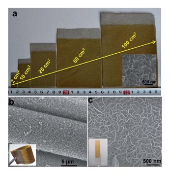
Fig. 5 (a) Photographs of NiFe-LDH nanoplatelet arrays synthesized on foam nickel substrates at various scales (inset: the SEM image of the NiFe-LDH sample on the 100 cm<sup>2</sup> substrate); synthesis time for all the samples is 300 s at room temperature. SEM images for the NiFe-LDH nanoplatelet arrays on (b) a conducting cloth and (c) FTO substrate (inset: their corresponding photographs).
