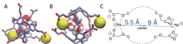
Fig. 8  $\text{Na}^+$  counter ions (yellow) near the  $m3n3$  cryptophane molecule in the absence of Xe ( $\lambda = 1$ ). (A) Top view. (B) Side view ( $90^\circ$  rotation of configuration in (A)). (C) Schematic illustration of counter ion coordination by the side chains.
