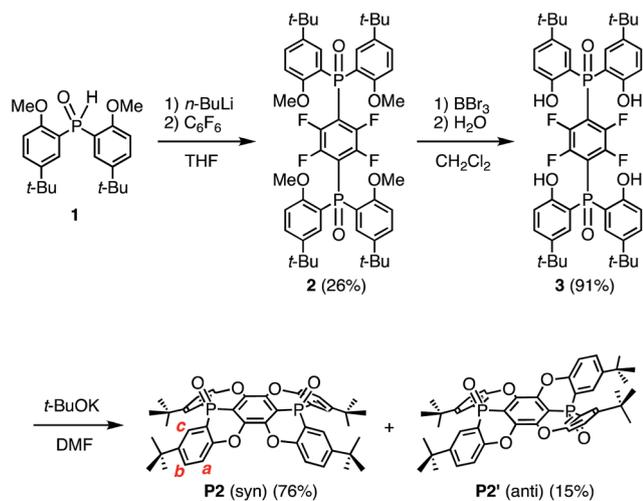
Scheme 1 Synthesis of bowl-shaped phosphorus-containing host **P2**.
