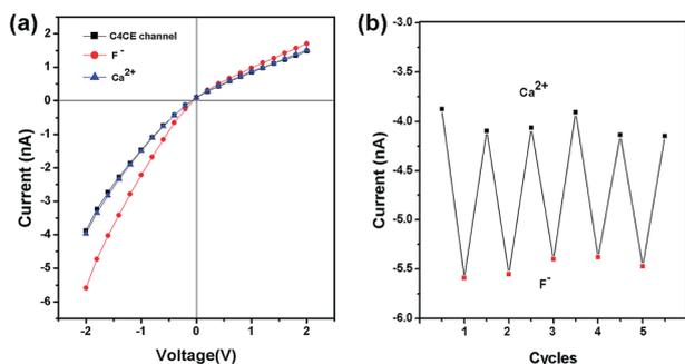
Fig. 5 The reversibility of the C4CE nanochannel. (a) The current change for the C4CE channel on addition and removal of  $\text{F}^-$ ; (b) the recyclability of the C4CE channel shown by the current change at  $-2$  V on addition and removal of  $\text{F}^-$ .
