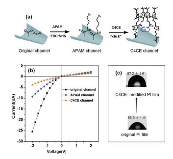
Fig. 2 The successful fabrication of the C4CE channel. (a) The construction process of the single conical nanochannel for F<sup>-</sup> sensing; (b) the changes in the I-V curve of the single nanochannel after each modification; (c) the contact angel on the flat film before and after modification of C4CE. These indicated that the C4CE host was modified successfully
