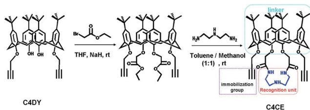
Scheme 1 The synthesis route of C4CE designed for F<sup>-</sup> sensing.
