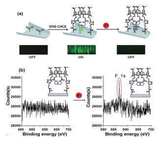
Fig. 4 (a) Laser scanning confocal microscopy (LSCM) images observed without DNS-C4CE, with DNS-C4CE and after immersing the DNS-C4CE-modified porous PI film in 10<sup>-3</sup> M F<sup>-</sup> solution: (b) the XPS spectra for the C4CE-modified film before and after immersion in  $10^{-3}$ M F<sup>-</sup> solution. These confirmed that the C4CE host can capture F<sup>-</sup>.
