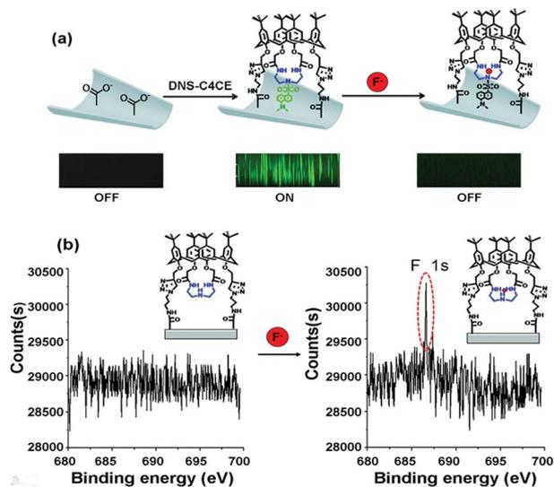
Fig. 4 (a) Laser scanning confocal microscopy (LSCM) images observed without DNS-C4CE, with DNS-C4CE and after immersing the DNS-C4CE-modified porous PI film in  $10^{-3}$  M  $F^{-}$  solution; (b) the XPS spectra for the C4CE-modified film before and after immersion in  $10^{-3}$  M  $F^{-}$  solution. These confirmed that the C4CE host can capture  $F^{-}$ .
