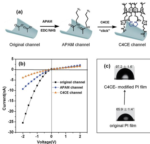
Fig. 2 The successful fabrication of the C4CE channel. (a) The construction process of the single conical nanochannel for  $\text{F}^-$  sensing; (b) the changes in the  $I$ - $V$  curve of the single nanochannel after each modification; (c) the contact angle on the flat film before and after modification of C4CE. These indicated that the C4CE host was modified successfully.
