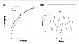
Fig. 5 The reversibility of the C4CE nanochannel. (a) The current change for the C4CE channel on addition and removal of  $F^-$ ; (b) the recyclability of the C4CE channel shown by the current change at -2 V on addition and removal of  $F^-$ .
