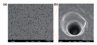
Fig. 1 (a) Scanning electron microscopy (SEM) image in track-etched PI film; (b) the enlarged image.
