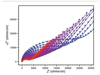
Fig. 3 Variable-temperature AC impedance spectra for **11a** taken from 300 K (blue points) to 373 K (red points) in 5 K intervals from 303 K on. Lines represent fit to an equivalent circuit diagram shown in the ESI.†
