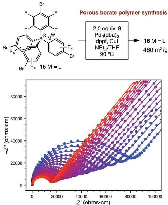
Scheme 3 Synthetic approach to porous polymer **16** and variable-temperature ac impedance spectra taken from 300 K (blue circles) to 373 K (red circles) in 5 K intervals from 303 K on. Lines represent fit to an equivalent circuit diagram shown in the ESI.†
