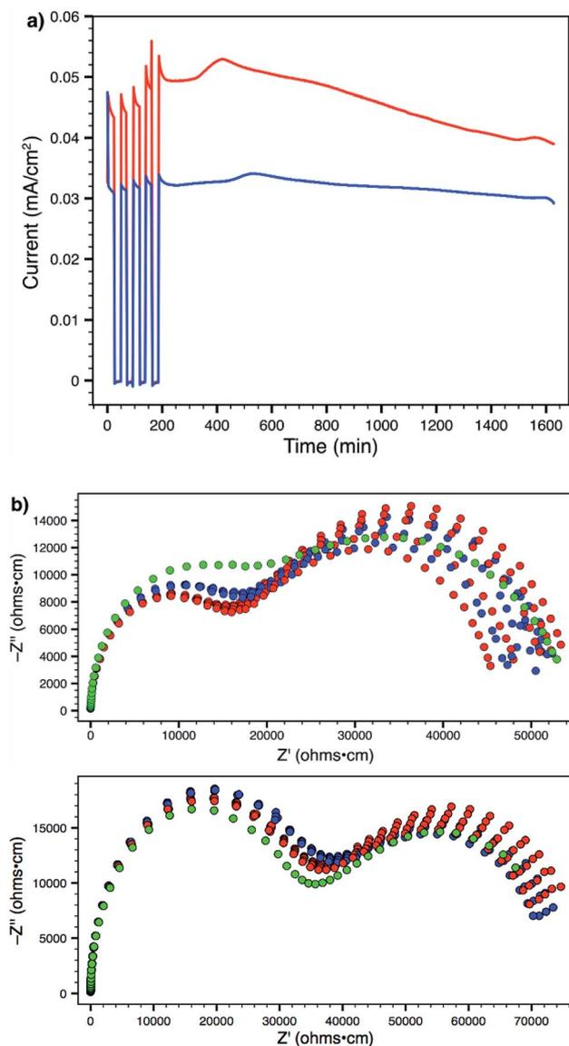
Fig. 7 (a) Current response from 300 mV applied potential to **14** (red) and **19** (blue) in a symmetric lithium metal cell. (b) AC impedance spectra collected during 24 hour operation of Li(s)|electrolyte|Li(s) symmetric cells. Top: Polymer **14**. Bottom: Polymer **19**. Red data represents impedance spectra taken without constant applied voltage. Blue data represents spectra taken with 300 mV applied voltage. Green data represents the final spectrum taken after the experiment.
