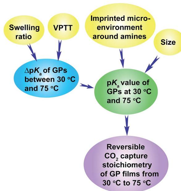
Scheme 3 Illustration of the design rationale for GPs that show large reversible CO<sub>2</sub> capture stoichiometry.
