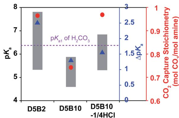
Fig. 2 p*K*<sub>a</sub> values (left Y-axis) at 75 °C (bottom of bar) and 30 °C (top of bar), and Δp*K*<sub>a</sub> values (blue right Y-axis, blue triangle) between 75 °C and 30 °C of **D5B2**, **D5B10**, and **D5B10-1/4HCl**, reversible CO<sub>2</sub> capture stoichiometries (red right Y-axis, red dot) of GP films in the temperature range 30–75 °C.
