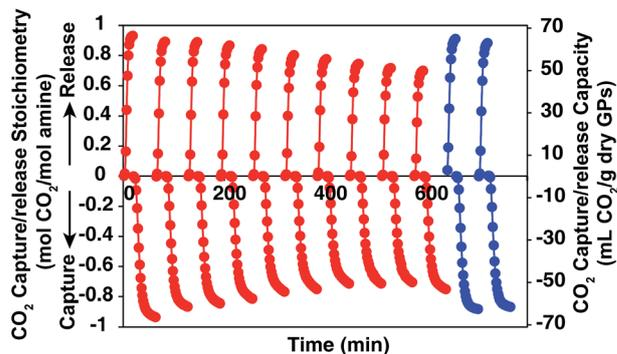
Fig. 7  $CO_2$  capture/release stoichiometry (right Y axis) and  $CO_2$  capture/release capacity (left Y axis) of GP D55B2T43 film with 4 mL water per g GPs. Red: first 10 cycles of  $CO_2$  release/capture by the GP film. After the first 10 cycles, 4 mL water per g GPs was supplied to the dried part of the GP film. Blue: the  $CO_2$  release-capture by the GP film after supplying 4 mL water per g GPs to the dried part of the GP film.
