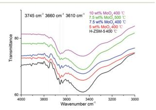
Fig. 4 Fourier transform-IR spectra of hydroxyl group regions on the parent H-ZSM-5 and MoO $_3$ -loaded samples prepared at 400 °C/500 °C.
