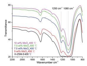
Fig. 5 Fourier Transform-IR spectra of H-ZSM-5 samples with different  $MoO_3$  loading levels prepared at  $400 \,^{\circ}\text{C}/500 \,^{\circ}\text{C}$ .
