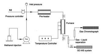
Fig. 1 Schematic representation of the reactor, and testing  $\boldsymbol{\vartheta}$  analysis system.
