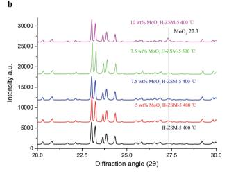
Fig. 2 (a) X-ray diffraction patterns ( $2\theta = 5-25^{\circ}$ ) of MoO<sub>3</sub>/ZSM-5 samples with various MoO<sub>3</sub> loadings and prepared at 400 °C/500 °C. (b) X-ray diffraction patterns ( $2\theta = 20-30^{\circ}$ ) of MoO<sub>3</sub>/ZSM-5 samples with various MoO<sub>3</sub> loadings and prepared at 400 °C/500 °C.
