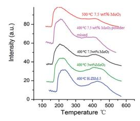
Fig. 6 NH $_3$ -temperature programmed desorption profiles of MoO $_3$ / H-ZSM-5 samples prepared via different conditions (impregnation/powder mixing, 400–500 °C) together with the original H-ZSM-5 sample (400 °C).
