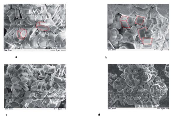
Fig. 7 (a) SEM image of the parent H-ZSM-5. (b) SEM image of H-ZSM-5 with 7.5 wt%  $MoO_3$ -400 °C dispersion. (c) SEM image of the parent H-ZSM-5 (post reaction). (d) SEM image of H-ZSM-5 with 7.5 wt%  $MoO_3$ -400 °C (post reaction).
