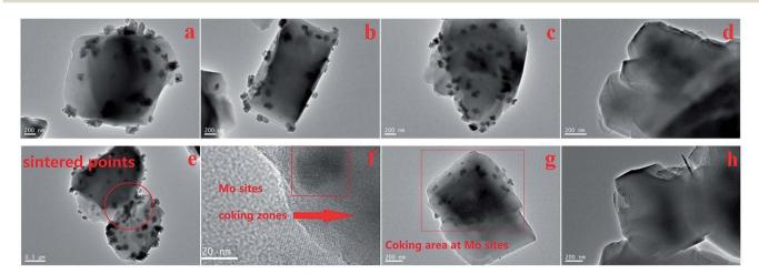
Fig. 8 TEM images of post catalytic-testing samples with different  $MoO_3$  loadings, (a) 5 wt%, (b) 7.5 wt%, (c) 10 wt% and (d) parent H-ZSM-5, (e) sintering effects (5 wt%), (f) amplified coking areas near the Mo species (5 wt%), (g) coking areas near Mo species (5 wt%) and (h) parent H-ZSM-5, all the samples are prepared at 400 °C and the MTH reaction proceeded at 400 °C More images of other samples are included in the Fig. S1–S9.†
