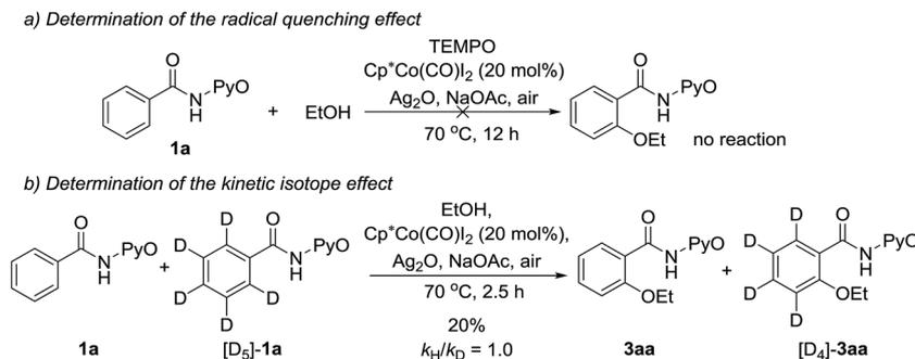
Scheme 15 Controlled experiments for  $\text{Co}^{\text{III}}$ -catalyzed  $\text{C}(\text{sp}^2)\text{-H}$  alkoxylation.
