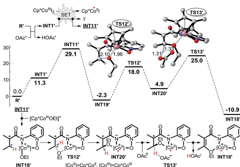
Scheme 16 The mechanism of  $\text{Cp}^*\text{Co}^{\text{III}}$  complex catalyzed  $\text{C}(\text{sp}^2)\text{-H}$  alkoxylation obtained at the M06-L(SMD, ethanol)/6-311++G(2df, 2pd)//SDD level (energy:  $\text{kcal mol}^{-1}$ , distance: Å).
