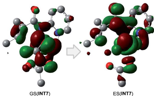
Fig. 2 The lowest excited-state doublet derives from excitation of an alpha electron from the singly occupied SOMO (GS(INT7)) into the nominally unoccupied LUMO (ES(INT7),  $d_{z^2}$ ). The resulting excited state is  $44.3 \text{ kcal mol}^{-1}$  above the ground state, corresponding to a photon energy of  $761.09 \text{ nm}$ .
