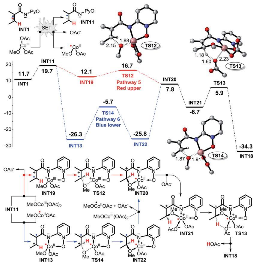
Scheme 10 Possible intermolecular SET pathways 5 (red, upper) and 6 (blue, lower) of Co<sup>III</sup>-catalyzed C(sp<sup>2</sup>)-H alkoxylation (energy: kcal mol<sup>-1</sup>, distance: Å).
