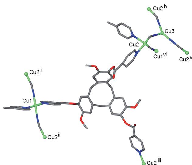
Fig. 1 Coordination geometries of Cu sites and ligand bridging behaviour from the crystal structure of complex **1**. Symmetry operators: (i)  $y, -x + y, 1 - z$ ; (ii)  $2/3 - y, 1/3 + x - y, 1/3 + z$ ; (iii)  $x - y, x, 1 - z$ ; (iv)  $-x + y, 1 - x, z$ ; (v)  $1 - y, 1 + x - y, z$ ; (vi)  $1/3 - x + y, 2/3 - x, z - 1/3$ .
