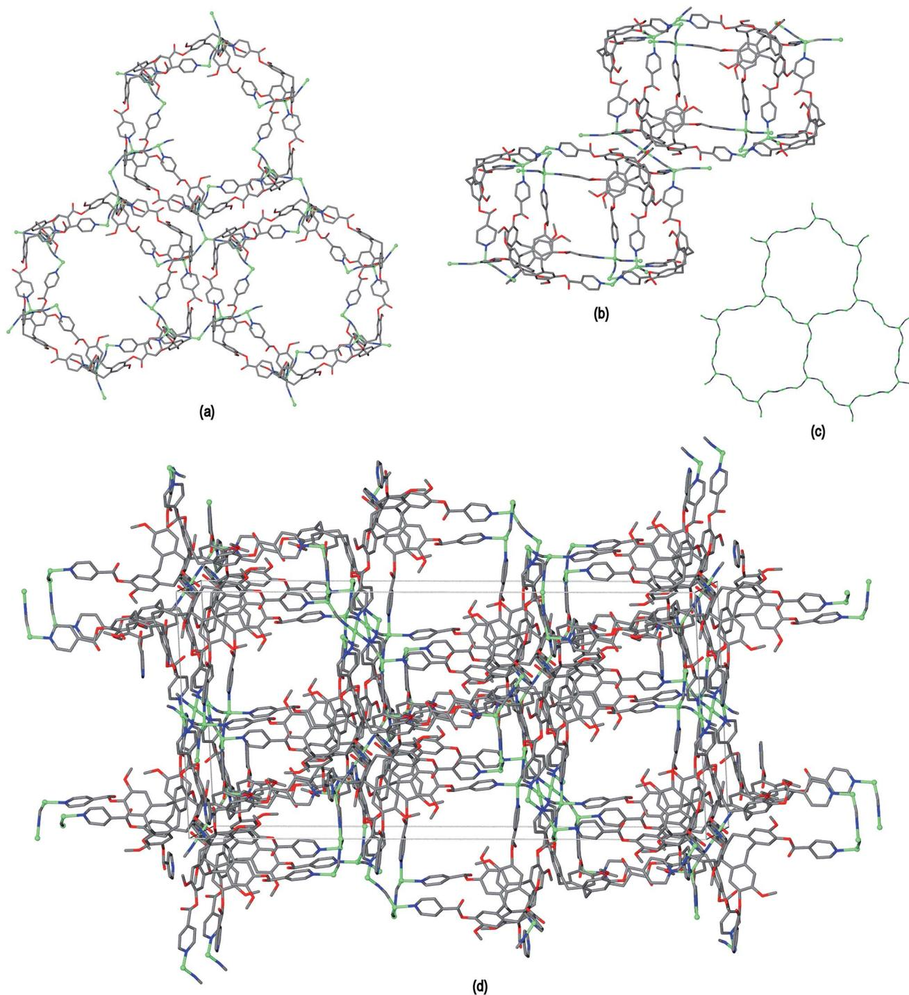
Fig. 2 Crystal structure of complex 1 illustrating the formation of hexagonal prism motifs within the 3D coordination polymer framework, (a) top view down the  $c$  axis of three prisms connected by a central  $\text{Cu}_3$  ion; (b) side view of two prisms from two different layers connected through  $\text{Cu-CN}$  bridges; (c) the copper cyanide expanded hexagonal net; (d) unit cell diagram viewed down the  $a$  axis.
