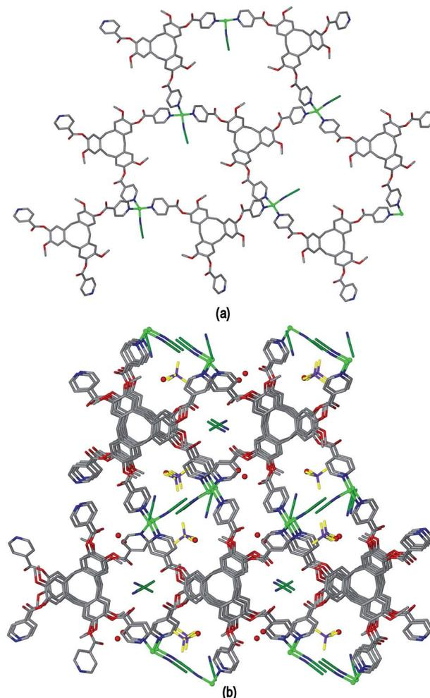
Fig. 10 Crystal structure of [Cu(L1)(NCMe)]·BF<sub>4</sub>·1.5(CH<sub>3</sub>CN)·2H<sub>2</sub>O **5**. (a) 2D Coordination polymer network with 6<sup>3</sup> topology; (b) packing diagram viewed down the *a* axis. Carbon atoms of CH<sub>3</sub>CN shown in dark green and H atoms excluded.
