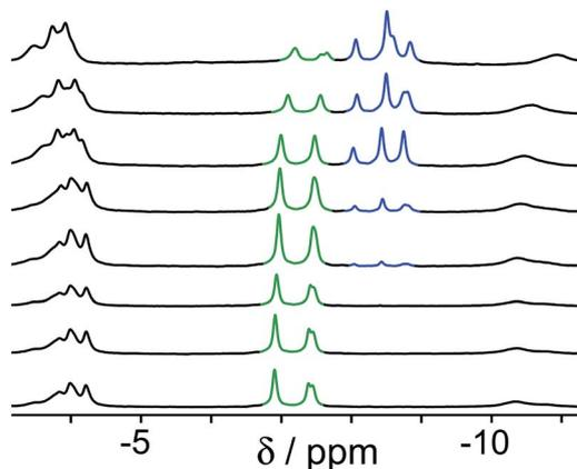
Fig. 4 Series of  $^1\text{H}$  NMR spectra ( $\text{D}_2\text{O}$ , 298 K) of a mixture of cage (0.2 mM), C (0.2 mM) and B (2.0 mM). pH values (from bottom to top): 5.0, 7.4, 8.9, 9.6, 9.8, 10.6, 11.3, 12.2. Replacement of bound C (green signals) by B (blue signals) as the pH rises is clear.
