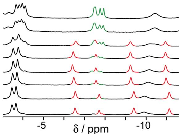
Fig. 3 Series of  $^1\text{H}$  NMR spectra ( $\text{D}_2\text{O}$ , 298 K) of a mixture of cage (0.2 mM), C (0.2 mM) and  $\text{H}_2\text{A}$  (0.98 mM). pH values (from bottom to top): 2.0, 4.1, 4.3, 4.6, 5.0, 5.6, 7.3, 8.8. Replacement of bound  $\text{H}_2\text{A}$  (red signals) by C (green signals) as the pH rises is clear.
