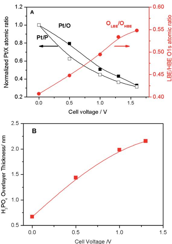
Fig. 3 (A) Pt/O and Pt/P atomic ratios normalized to the corresponding values at the OCV (black left-hand-side axis), and LBE ( $\text{O}_{\text{LBE}}$ ) to HBE ( $\text{O}_{\text{HBE}}$ ) oxygen intensity (red right-hand-side axis) obtained via deconvolution of spectra presented in Fig. 2B as a function of the cell voltage. (B) Apparent thickness of the PA film calculated as a function of the applied cell voltage.
