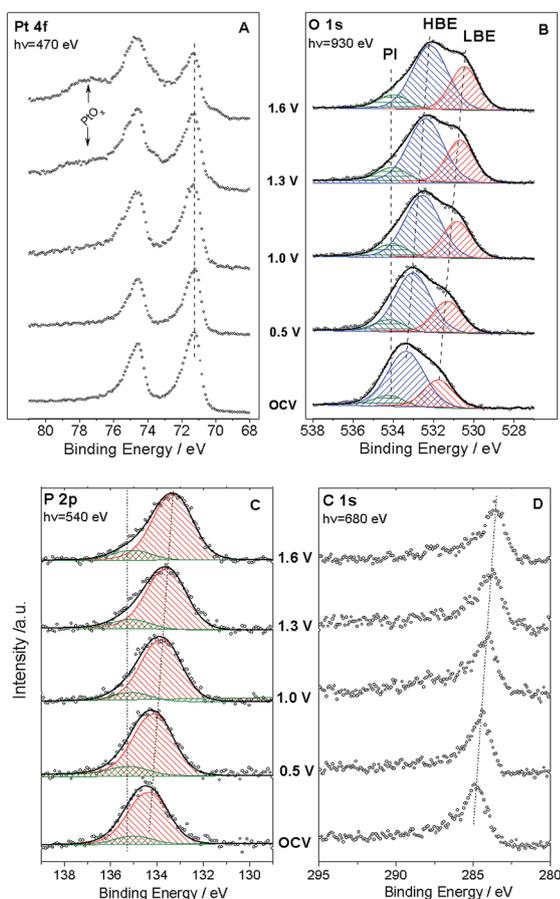
Fig. 2 Pt 4f (A), O 1s (B), P 2p (C), and C 1s (D) spectra acquired *in situ* under 0.3 mbar  $\text{H}_2\text{O}$  and  $180^\circ\text{C}$  at various cell voltages. Panels B and C also show the results of the O 1s and P 2p spectra deconvolution. See text for details.
