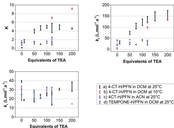
Fig. 4 Average values of the equilibrium constants ( $K$ ) and forward ( $k_f$ ) and reverse ( $k_r$ ) rate constants as a function of triethylamine (TEA) base added for (a) the PFN-5/4-CT-H reaction in dichloromethane at 25 °C, (b) the same reaction at 10 °C, (c) the same reaction in acetonitrile at 25 °C, and (d) for the PFN-5/TEMPONE-H control reaction in dichloromethane at 25 °C. The error bars are the calculated standard deviations of replicate samples.
