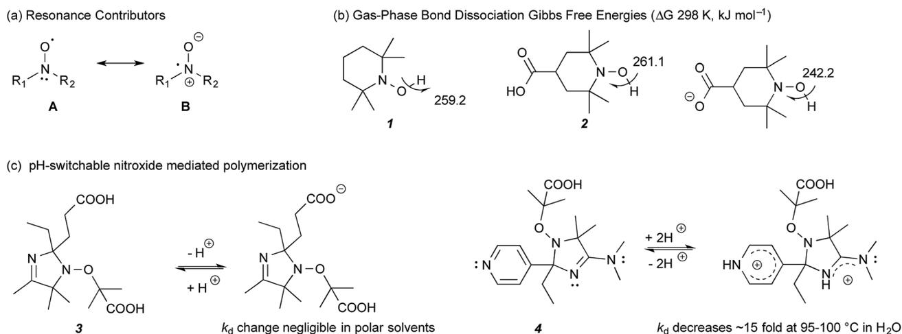
Fig. 1 (a) Resonance contributors of a nitroxide radical. (b) Calculated bond dissociation Gibbs free energies (298 K,  $\text{kJ mol}^{-1}$ ) of non-substituted TEMPO-H (**1**) and protonated and deprotonated 4-CT-H (**2**) at 25 °C.<sup>9</sup> (c) Literature studied pH-switchable nitroxides.<sup>10</sup>
