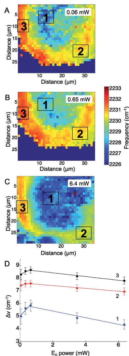
Fig. 4 The observed CN stretch frequency of *p*-mercaptobenzonitrile on a roughened silver surface is plotted at increasing incident laser power: (A) 0.06 mW, (B) 0.65 mW, and (C) 6.4 mW. (D) The average frequency shift observed in each region of interest (ROI) was plotted against the incident laser power ( $E_0$ ). The lines in D are guides for the eye.
