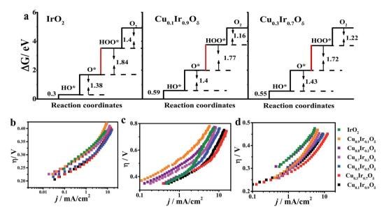
Fig. 7 (a) Standard free energy diagram for the OER in IrO<sub>2</sub>,  $Cu_{0.1}Ir_{0.9}O_{\delta}$  and  $Cu_{0.3}Ir_{0.7}O_{\delta}$ . (b-d) Tafel plots in acidic, neutral and basic solutions, respectively. The curves are iR-corrected in the acidic ( $\sim$ 18  $\Omega$ ), neutral ( $\sim$ 15  $\Omega$ ) and basic ( $\sim$ 28  $\Omega$ ) solutions, respectively. The catalyst mass loading was  $\sim$ 0.2 mg cm<sup>-2</sup> for all electrodes.
