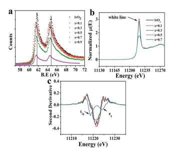
Fig. 5 (a) XPS spectra of Ir-4f in  $Cu_xIr_{1-x}O_\delta$  compositions. The solid vertical lines correspond to the Ir-4f $_{7/2}$  and 4f $_{5/2}$  peak positions of Ir $O_2$ . (b) Normalized Ir- $L_{III}$  edge XANES spectra for  $Cu_xIr_{1-x}O_\delta$  compositions. (c) Second derivatives of Ir- $L_{III}$  edge XANES spectra for  $Cu_xIr_{1-x}O_\delta$  compositions.
