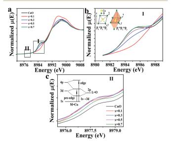
Fig. 3 (a) Normalized Cu-K edge XANES spectra for  $Cu_xIr_{1-x}O_{\delta}$ compositions. (b) Shows the shakedown transition and the inset is a diagram of the Cu-4p orbital energy in two different symmetries. (c) Shows the amplified pre-edge region and the inset diagram shows the energy level of possible transitions. (b) and (c) correspond to the selected areas, I and II, in (a),
