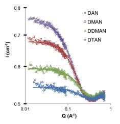
Fig. 1 Scattering patterns of 5 wt% dodecylammonium nitrate surfactants in EAN at 60  $^{\circ}\text{C}.$
