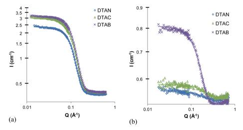
Fig. 4 SANS pattern of 5 wt% dodecyltrimethylammonium chloride, bromide and nitrate in (a) EtAN and (b) EAN at 60 °C.
