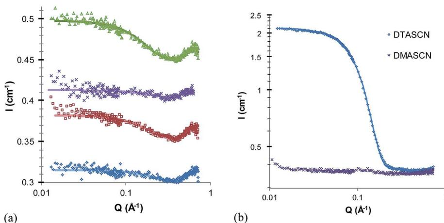
Fig. 3 (a) Stack plot, vertical offset of +0.05 for each plot, of scattering patterns of 5 wt% solutions dodecylammonium thiocyanate surfactant in EASCN at 60 °C. DASCN  $\Delta$ , DMASCN  $\times$ , DDMASCN  $\square$ , DTASCN  $\diamond$ . (b) Scattering patterns of 5 wt% solutions dodecylammonium thiocyanate surfactants in EtASCN at 60 °C, note no scattering pattern was collected of DASCN due to low solubility.
