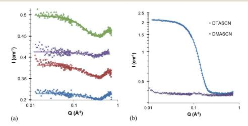
Fig. 3 (a) Stack plot, vertical offset of +0.05 for each plot, of scattering patterns of 5 wt% solutions dodecylammonium thiocyanate surfactant in EASCN at 60 °C. DASCN  $\triangle$ , DMASCN  $\times$ , DDMASCN  $\times$
