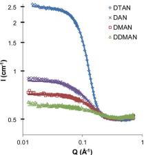
Fig. 2 Scattering patterns of 5 wt% dodecylammonium nitrate surfactants in EtAN at 60  $^{\circ}$ C.
