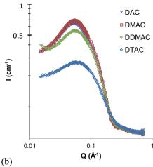
Fig. 6 Scattering of 1 wt% dodecylammonium (a) nitrate and (b) chloride surfactants in water at 60 °C.
