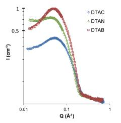
Fig. 5 Scattering patterns of quaternary ammonium surfactants in water at 25  $^{\circ}\text{C}.$
