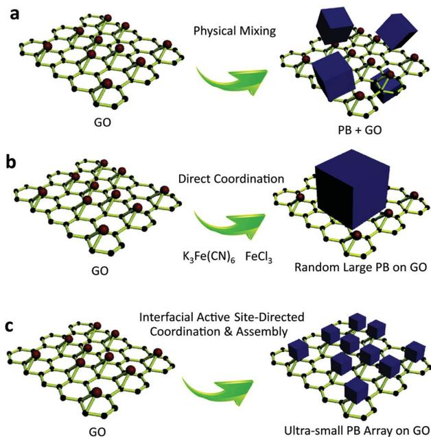
**Fig. 1** Comparison of the classic physical mixing, direct coordination, and interfacial site-directed growth approaches for sub-5 nm porous Prussian blue nanocrystals. (a) Mixture of Prussian blue and graphene oxide resulting from the physical mixing method. (b) Random large Prussian blue growth on graphene oxide by the direct coordination method. (c) Ultra-small porous Prussian blue assembly arrays on graphene resulting from the interfacial site-directed growth method.
