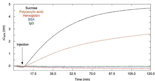
**Fig. 2** Diffusion of sucrose (MW = 342 Da), poly(acrylic acid) (MW = 2 kDa), hemoglobin (MW = 64.0 kDa), BSA (MW = 66.4 kDa) and IgG (MW = 150 kDa) through the microporous membrane of 0.4  $\mu\text{m}$  pore size (concentration of 10 mg mL<sup>-1</sup> for sucrose and poly(acrylic acid) solution and 1 mg mL<sup>-1</sup> for each protein solution).
