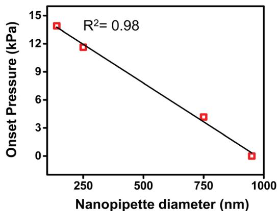
Fig. 3 Plot of onset pressure (obtained from  $X$ -axis intercept of Fig. S4<sup>†</sup>) versus tip diameter.
