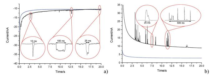
Fig. 4 Representative chronoamperometric scans in a  $5.9 \times 10^{-13}$  mol dm $^{-3}$  suspension using a cylindrical carbon fibre wire electrode at a potential of (a) -1.20 V (vs. SCE); (b) +1.20 V (vs. SCE). Blue line: blank scan in 0.1 M KCl with 50 mM KH $_2$ PO $_4$ , 50 mM K $_2$ HPO $_4$  (PBS) buffer solution mentioned in the Experimental section. Black line:  $5.9 \times 10^{-13}$  mol dm $^{-3}$  graphene nanoplatelet (GNP) suspension scan showing capacitative impacts.
