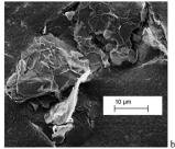
Fig. 2 SEM images of the graphene platelets used in this work.
