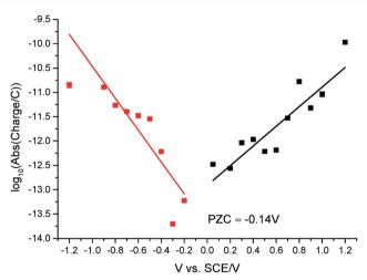
Fig. 6  $5.9 \times 10^{-13}$  mol dm<sup>-3</sup> suspension impacts with absolute charge of nanoparticle impacts in logarithmic (log10) scale plotted against applied potential (vs. SCE). Red squares: values with applied potential < 0 V; black squares: values with applied potential > 0 V (vs. SCE). The intersection potential of the two lines is used to estimate the PZC value of GNPs, where PZC is determined to be -0.14 V (vs. SCE).
