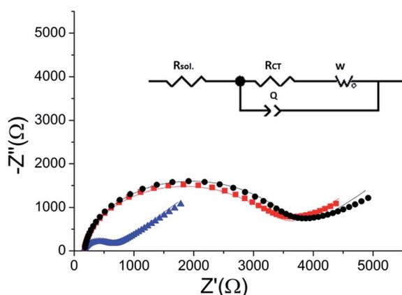
Fig. 5 Reversibility of the phosphorylation – dephosphorylation process. Black (●) – the  $R_{CT}$  of the peptide monolayer ( $R_{CT} = 3400 \Omega$ ). Blue (▲) – the  $R_{CT}$  of the monolayer following phosphorylation with ERK2 ( $R_{CT} = 474 \Omega$ ). Red (■) – the impedance of the monolayer after dephosphorylation with AP ( $R_{CT} = 3250 \Omega$ ). Lines – fits to the equivalent circuit (inset).
