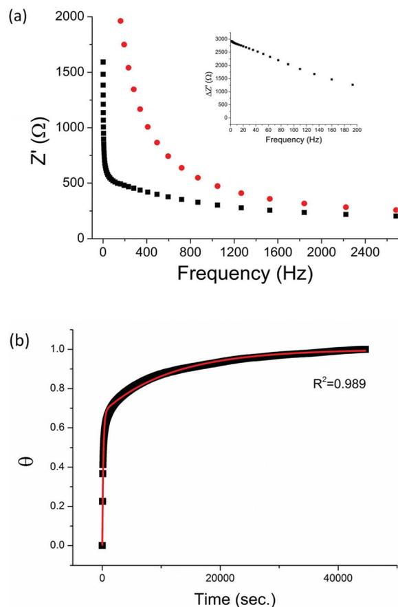
Fig. 3 (a) Bode plots of a clean gold electrode (black square) and the same electrode after peptide adsorption overnight (red circle). Inset: the difference in the real impedance ( $Z'$ ) between the peptide coated electrode and the clean gold electrode ( $\Delta Z'$ ). (b) Adsorption of HDGF 160–174 onto a clean gold electrode. Relative surface coverage ( $\theta$ ) was plotted against time ( $\blacksquare$ ). The curve was fit to a second order reaction kinetic equation (red line).
