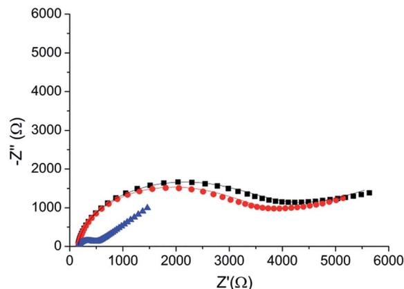
Fig. 6 A phosphorylation process with CaMK2. Black (■) – the  $R_{CT}$  of the peptide monolayer ( $R_{CT} = 4080 \Omega$ ). Red (●) – the  $R_{CT}$  of the monolayer following phosphorylation with CaMK2 ( $R_{CT} = 3600 \Omega$ ). Blue (▲) – the  $R_{CT}$  of the monolayer after phosphorylation with ERK2 ( $R_{CT} = 390 \Omega$ ). Lines – fits to the equivalent circuit.
