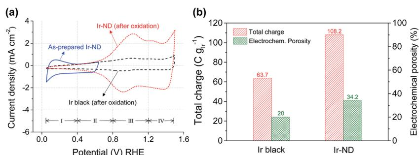
Fig. 3 Surface redox electrochemistry of commercial iridium black and iridium nanodendrites (Ir-ND): (a) cyclic voltammograms (CVs) of as-prepared and oxidized nanodendrites. Conditions: 25 °C, N<sub>2</sub>-purged 0.05 M H<sub>2</sub>SO<sub>4</sub>, 20 mV s<sup>-1</sup>. The CV of the as-prepared Ir nanodendrites (Ir-ND) was recorded between +0.05 to +0.64 V<sub>RHE</sub> to avoid Ir oxide formation. (b) Electrochemical total charge and porosity of Ir-ND and Ir black.
