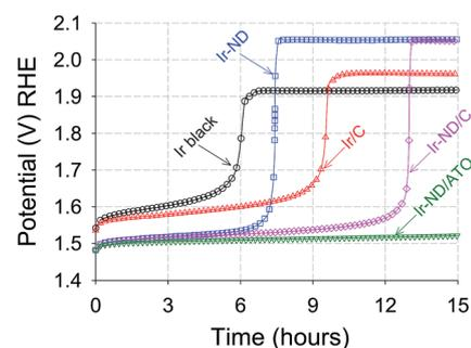
Fig. 7 Accelerated constant current-load durability test (ADT) of Ir-ND OER electrocatalysts in comparison to reference catalysts measured under identical conditions. test time: 15 h, N<sub>2</sub>-purged condition, catalyst loading:  $10.2 \mu\text{g}_{\text{Ir}} \text{ cm}^{-2}$ , 1600 rpm,  $10 \text{ mA cm}^{-2}$ .
