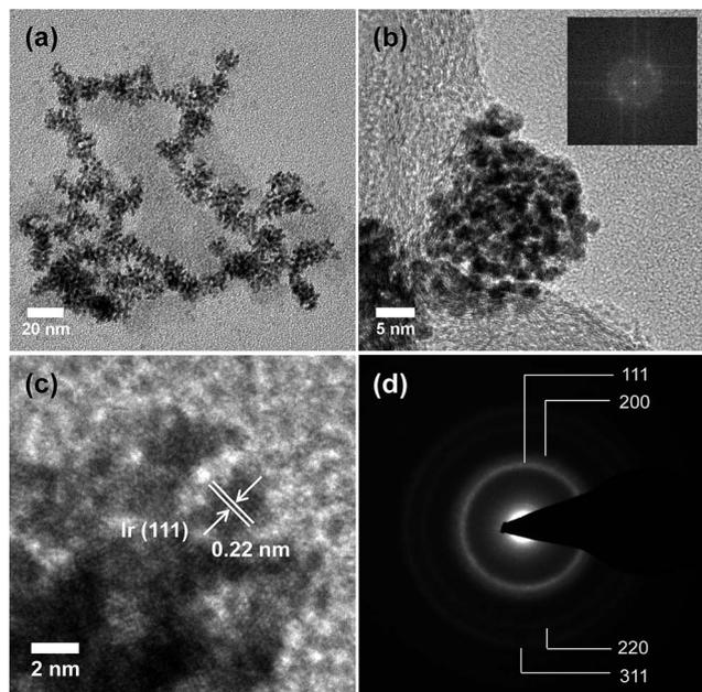
Fig. 1 (a) Low and (b) high resolution TEM images of the Ir nanodendrites (Ir-ND) synthesized by reducing H<sub>2</sub>IrCl<sub>6</sub>·xH<sub>2</sub>O with NaBH<sub>4</sub> in the presence of TTAB and the corresponding Fourier-transform (FT) pattern of the Ir-ND (inset b). (c) Magnified HRTEM image of one single Ir-ND and (d) the corresponding SAED pattern.
