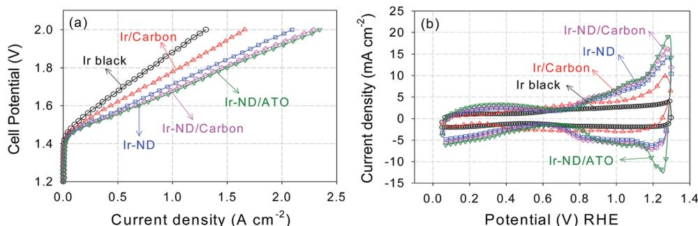
Fig. 6 Electrocatalytic performance of Ir-ND catalysts in a single PEM electrolyzer cells: (a) Membrane Electrode Assembly (MEA) polarization curves with a catalyst loading of  $1.0 \text{ mg cm}^{-2}$  and (b) cyclic voltammograms,  $50 \text{ mV s}^{-1}$ . Other conditions:  $80 \text{ }^\circ\text{C}$  cell temperature,  $5 \text{ cm}^2$  active electrode area, preheated  $80 \text{ }^\circ\text{C}$  deionized water was supplied at  $1.5 \text{ mL min}^{-1}$ .
