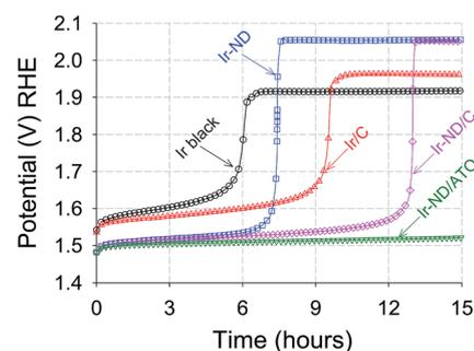
Fig. 7 Accelerated constant current-load durability test (ADT) of Ir-ND OER electrocatalysts in comparison to reference catalysts measured under identical conditions. test time: 15 h, N<sub>2</sub>-purged condition, catalyst loading: 10.2 μg<sub>Ir</sub> cm<sup>-2</sup>, 1600 rpm, 10 mA cm<sup>-2</sup>.
