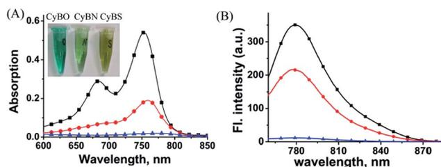
Fig. 1 The absorption (A) and fluorescence (B) spectra of the compounds **CyBO** (■), **CyBN** (●), and **CyBS** (▲) (10  $\mu\text{M}$ ) in pH = 7.4, PBS/DMF = 95/5. The excitation wavelengths are at 746 nm for **CyBO**, 745 nm for **CyBN**, and 748 nm for **CyBS**, respectively. Inset: (A) the visual colors of the **CyBX** dyes (left to right: X = O, N, and S) in PBS aqueous solution.
