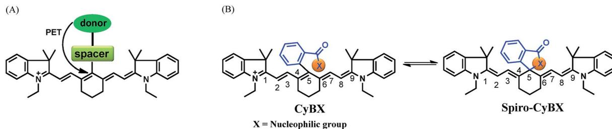
**Scheme 1** Design strategy for the new NIR functional **CyBX** ( $X = \text{O}, \text{N},$  or  $\text{S}$ ) dyes with an intrinsic spiro-cyclization based mechanism which modulates fluorescence On–Off. (A) The traditional PET mechanism for tuning fluorescence of heptamethine cyanines. (B) The spiro-cyclization based process of the novel functional NIR **CyBX** dyes described in this work.
