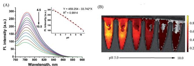
Fig. 5 (A) pH-dependence of the fluorescence spectra of the NIR probe CyBN (10  $\mu$ M, PBS/DMF: 95/5) upon excitation at 745 nm. Inset: plot of the fluorescence intensity versus pH. (B) The fluorescent images of CyBN (10  $\mu$ M, DMF/PBS 5/95) at pH 5.0 to 10.0 using the IVIS Lumina XR (IS1241N6071) *in vivo* imaging system with an excitation filter of 675 nm and an emission range of 760–810 nm.
