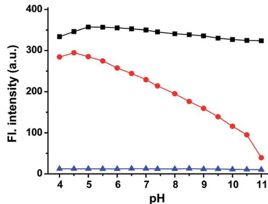
Fig. 2 The maximum emission intensity of the compounds: **CyBO** (■), **CyBN** (●), and **CyBS** (▲) (10  $\mu\text{M}$ , pH = 7.4, PBS/DMF = 95/5) at various pH values. The excitation wavelengths are at 746 nm for **CyBO**, 745 nm for **CyBN**, and 748 nm for **CyBS**, respectively.
