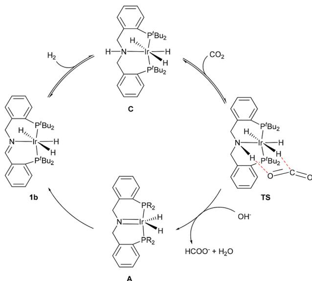
Scheme 2 Proposed mechanism for the hydrogenation of CO<sub>2</sub> catalyzed by **1b**.
