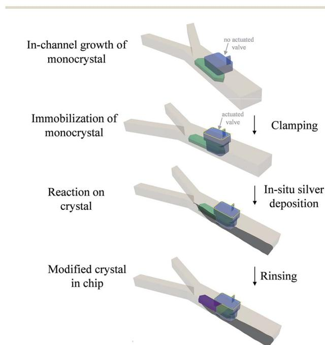
**Scheme 1** The route used for the modification of crystals in a fluid channel with pneumatic clamps for immobilizing and masking and area of it. The green object represents the original crystal grown in the chip, the purple area the modified material and the light green area an intermediate zone where partial reaction could take place.
