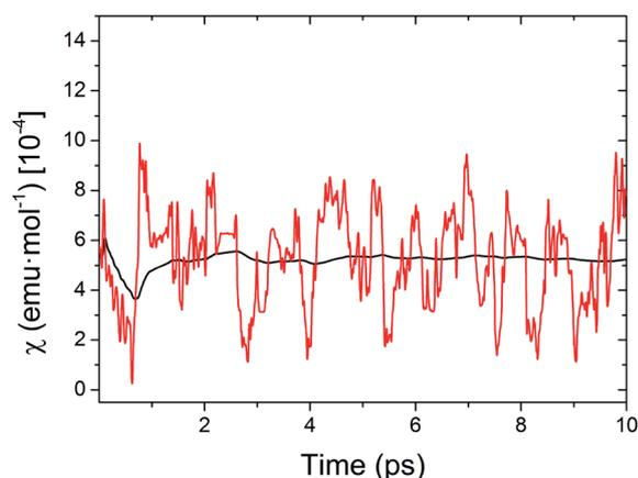
**Fig. 8** Time-resolved fluctuations of the sampled values of  $\chi$  along the AIMD trajectory (red curve) and evolution of the computed cumulative running average of  $\chi$  (black curve) for the HT phase of TTTA at 300 K.
