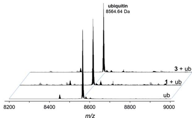
Fig. 4 Deconvoluted nESI-Q-TOF mass spectra of ubiquitin (8564.64 Da) and after incubation with **1** or **3** for 24 h. The mixture was incubated at a 2 : 1 metal-to-protein ratio in tetramethylammonium acetate.
