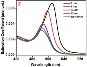
Fig. 3 Near-field distribution of two-photon scattering or second-harmonic intensity for nano-antenna with different spacing: (A) 3 nm, (B) 5 nm, (C) 10 nm and (D) 22 nm. (E) Simulated extinction spectra for monomer and nano-antenna with different spacing.
